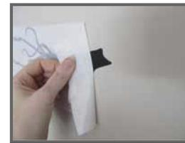
9) Slowly pull back the masking layer at a 180° angle. If the graphic starts to peel up, re-burnish and try again.
